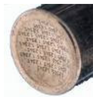
Bullet with engraved tracking number
